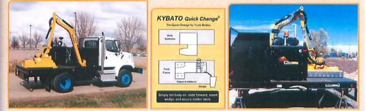
Remove the Tiger TrucKat in minutes with the use of the patented Kybato Quick Change system. The quick disconnect system allows the truck to be used for other applications throughout the year.
